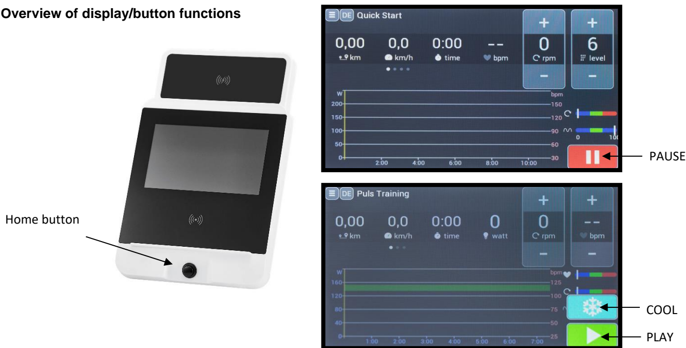
Fig. 2: Monitor view, to explain the button functions, actual view may vary in colour, button assignment is the same.
